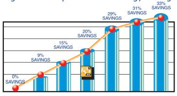
60 AFUE 64 AFUE 70 AFUE 80 AFUE 90 AFUE 92 AFUE 95 AFUE Percentage based on national averages; may vary according to efficiency of current unit and installation.
